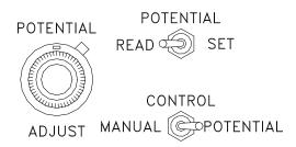
1. With the Manual-Potential Control switch in the Manual position, increase link bars to obtain an output slightly higher than required, but still within the rating of the rectifier.
